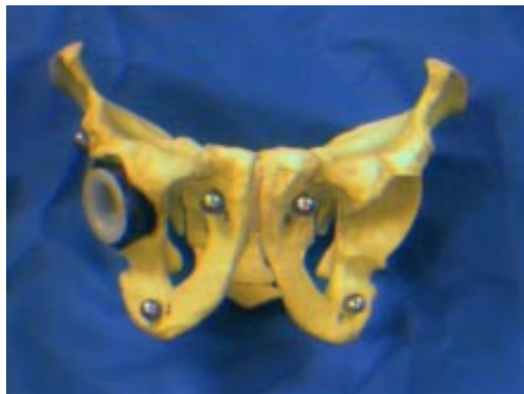
Figure 3. Pelvis phantom with implant used as model in usability experiment. Note fiducial spheres.
